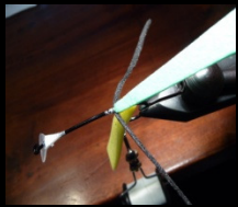
Tie the bottom and top Segment, then the side Striping
