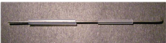
Cut the 1/8" OD plastic tubing into a piece 1" long. Cut the 3/32" OD plastic tubing into a piece 5/8" long. Insert the tube fly mandrel into the pieces of tubing to hold them in alignment while inserting them together.
